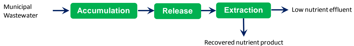
Figure 31: Three-Step Framework for Enabling Extractive Nutrient Recovery from Dilute Wastewater (Latimer et al., 2015a)
