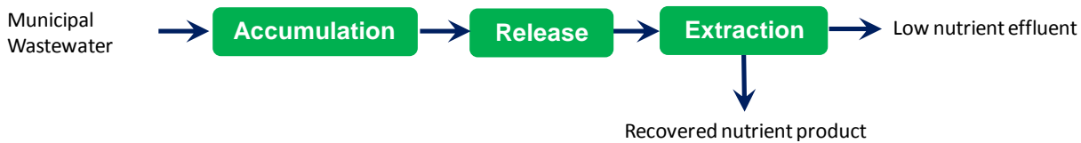
Figure 26: Integrated approach for implementing extractive nutrient recovery in WRRFs (Latimer et al., 2012a)
